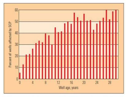
SCP=Sustained Casing Pressure. Also called sustained annular pressure in one or more of the casing annuli.
